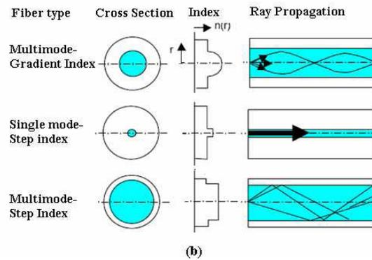
Figure 3. Different types of optical fibers.
