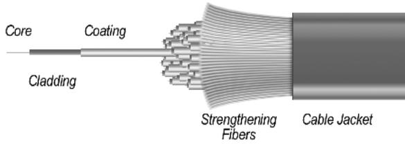
Figure 1. Basic structure of an optical fiber.
