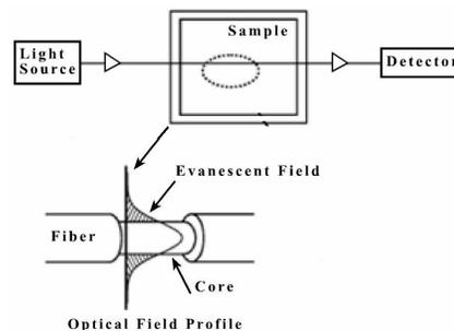
Figure 7. Evanescent wave fiber optic chemical sensor.
