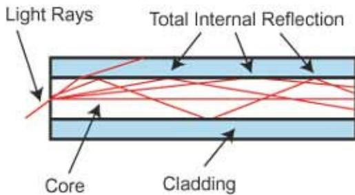
Figure 2. Total internal reflection in an optical fiber.
